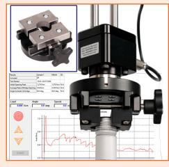
An adjustable Stelvin® cap mandrel ensures optimum accuracy in torque measurement
